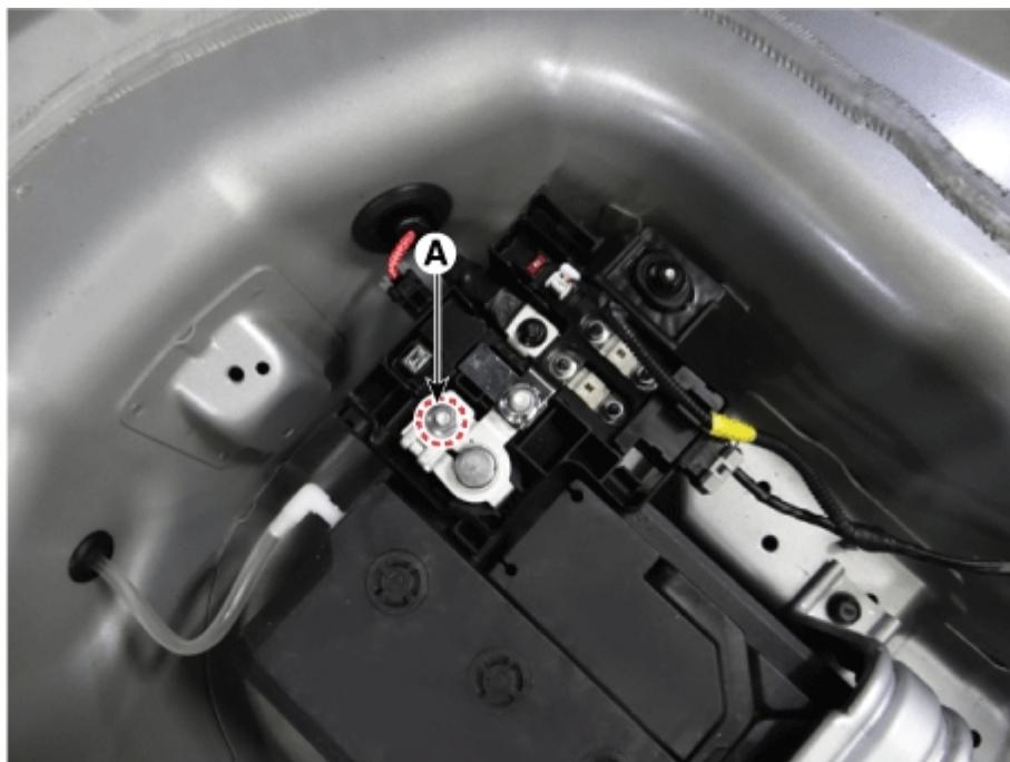
If battery positive connection is loose, disconnect ground(GND) cable first before attempting to remove or tighten plus connection, to prevent personal injury.
