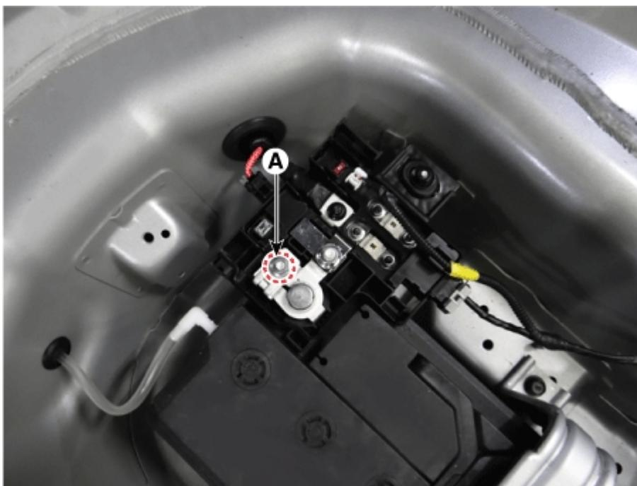
3. If the battery clamp on battery negative (-) terminal is not seated securely:
